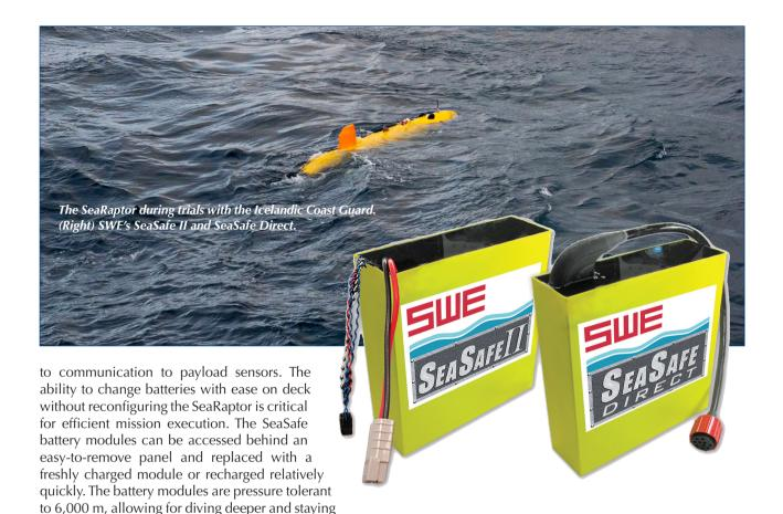
During the testing operations on the Icelandic Coast Guard Vessel *Pór*, the SeaRaptor carried out 10 hr. of surveys in shallow and deepwater to validate the sensor performance and navigational accuracy. For continuous surveying, the battery modules can be hot swapped in 20 min. While the AUV is in the water, the battery modules can be recharged over a period of about 4 hr. The SeaRaptor performed flawlessly during the testing operations, locating the wings of a B-24 bomber of the 1940s.
