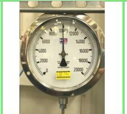
Pressure test Guage at 10K psig for 6 hours
