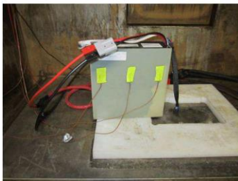
T5 – External Short Circuit
