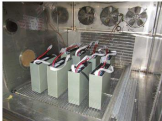
T5 – External Short Circuit
