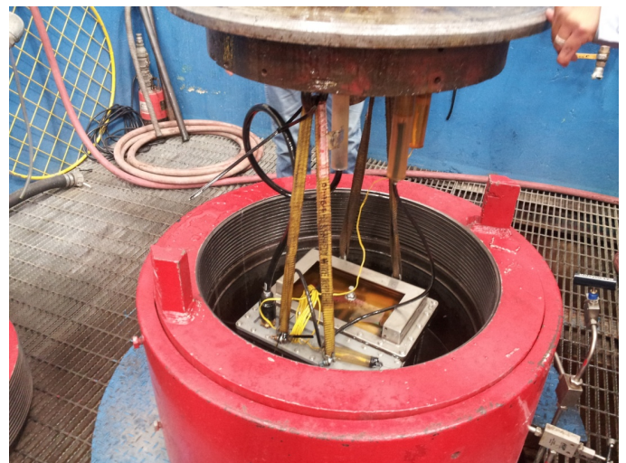
Figure 5. SeaSafe Case Being Lowered Into Pressure Test Chamber
