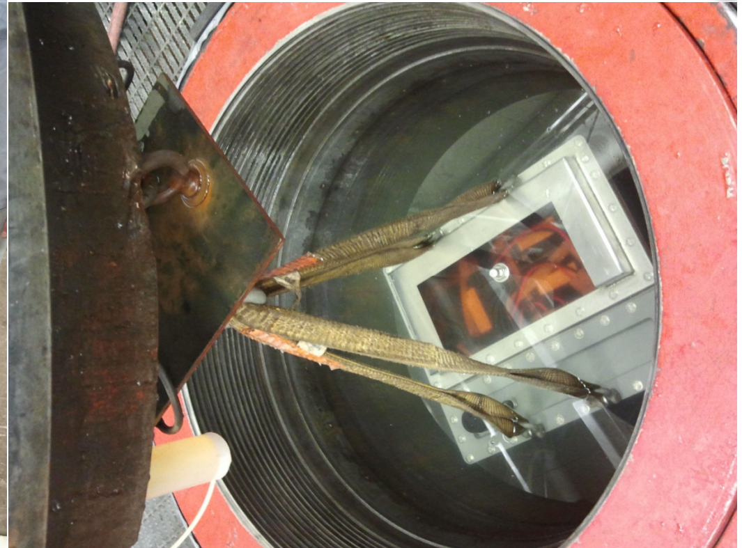
Measuring in-water weight of Battery System Prior to Pressure Testing.
