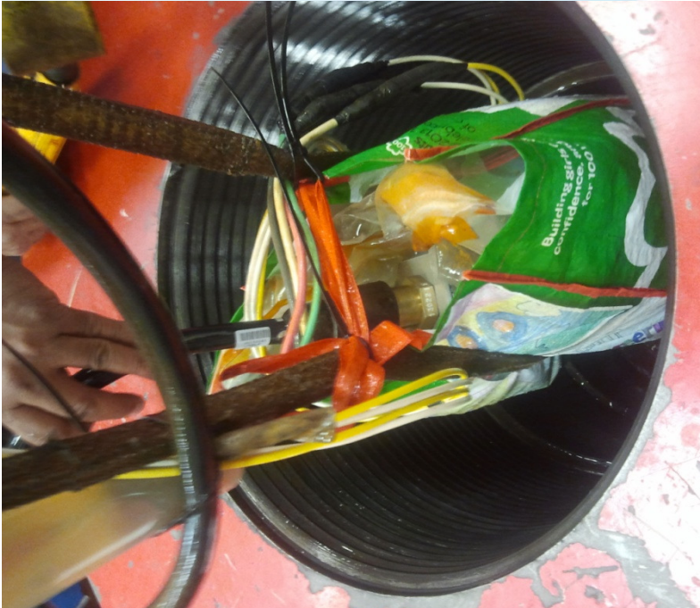
Cells Carried in Girl Scout Tote Bag Being Lowered Into Pressure Test Chamber.
