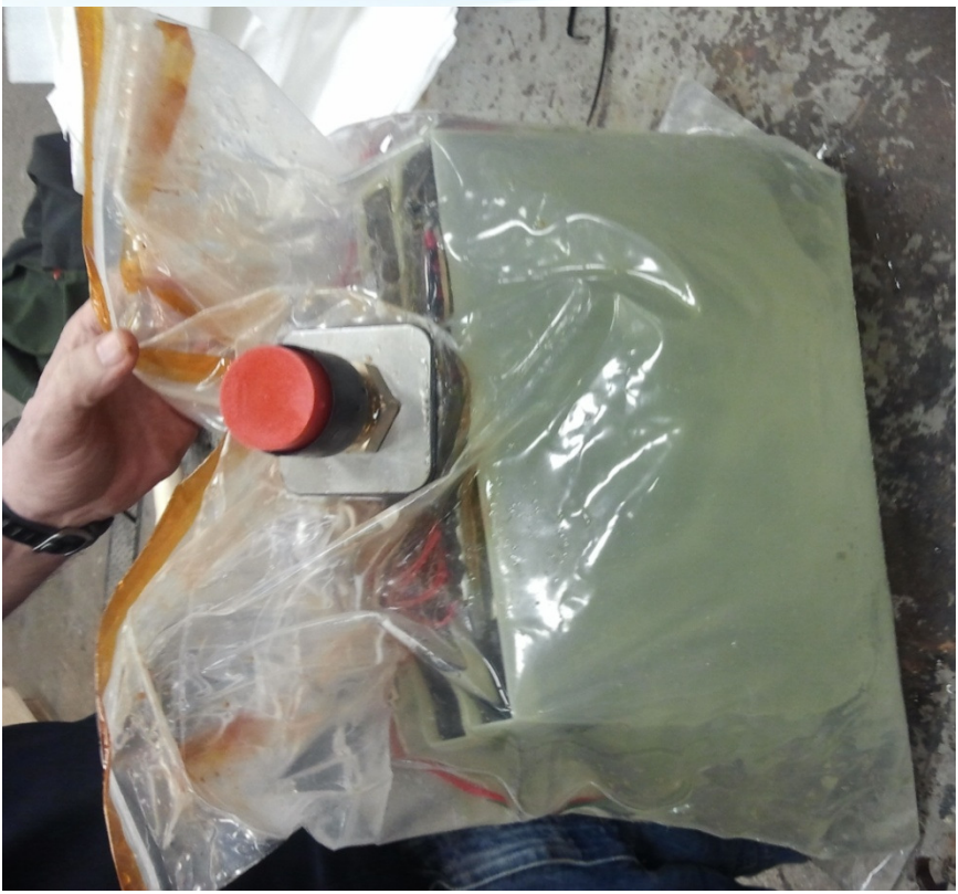
Two Cells Bagged and Filled w/Mineral Oil Prior to Pressure Testing.
