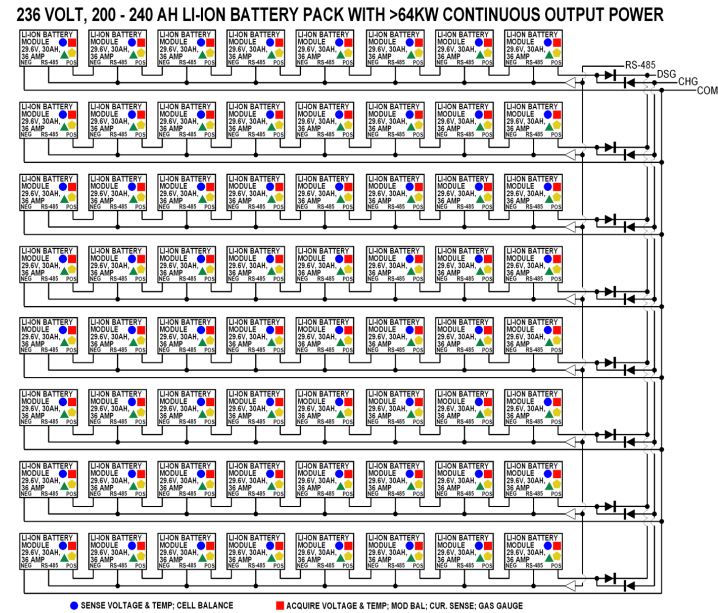
Figure 3. Example Distributed Architecture Lithium-Ion Battery System
